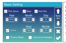
Factory Reset: Reset all parameters of the inverter. Lock out all changes: Enable this menu for setting parameters that require locking and cannot be set up. Before performing a successful factory reset and locking the systems, to keep all changes you need to type in a password to enable the setting.
