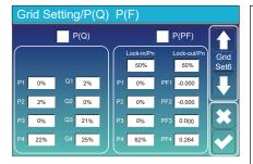
**P(Q):** It is used to adjust the inverter reactive power according to the set active power. **P(PF):** It is used to adjust the inverter PF according
