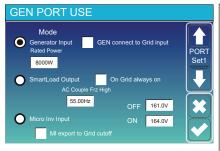
Generator input rated power: allowed Max. power from diesel generator.
