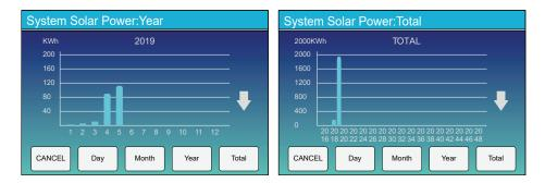
Solar power curve for daily, monthly, yearly and total can be roughly checked on the LCD, for more accuracy power generation, pls check on the monitoring system. Click the up and down arrow to check power curve of different period.
