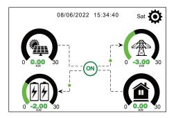
1. The icon in the center of the home screen indicates that the system is Normal operation. If it turns into "comm./F01~F64", it means the inverter has communication errors or other errors, the error message will display under this icon(F01-F64 errors, detail error info can be viewed in the System Alarms menu).
