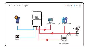
The 1st priority power of the system is always the PV power, then 2nd and 3rd priority power will be the battery bank or grid according to the settings. The last power backup will be the Generator if it is available.
