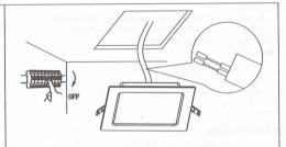
2.Switch OFF the power before starting the installation
