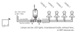
b. A one-gang wireless switch controls | c. A two-gang wireless switch a wireless receiver
