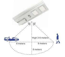
Mode 1: Press induction button to make it enter into sensor mode when object walk into the detective area lights turn on automatically; when object walk out of the detective area, 15 seconds later, lights keep 20% brightness. Mode 2: Light will turn on all the time
