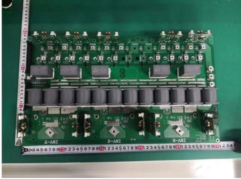
Boost-Inverter board (Components side)
