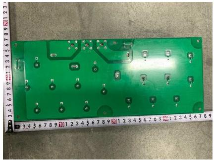
Capacitor board(Soldered side)
