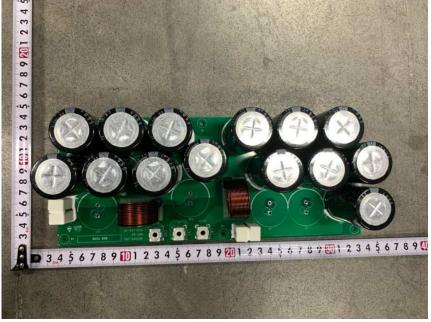
Capacitor board(Components side)
