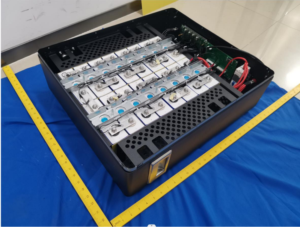
Figure 5 Inside view of battery
