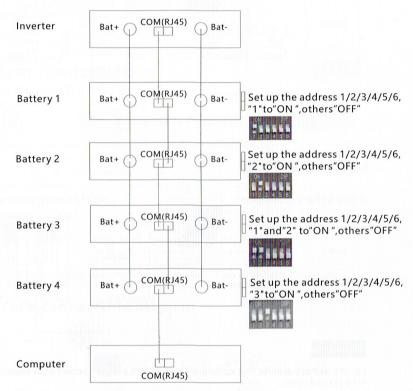
Use the computer software to monitor the battery data
