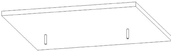
1. Drill holes on the wall, and plug the expansion sleeve into the holes
