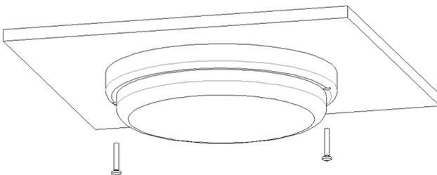
3. Align with the hole position and fix the lamp body with screws
